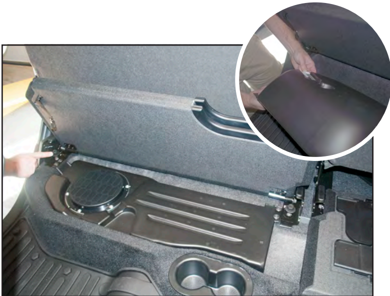
1. Fold rear seat upwards to remove the (8) 18 mm bolts from the underside of seat.
